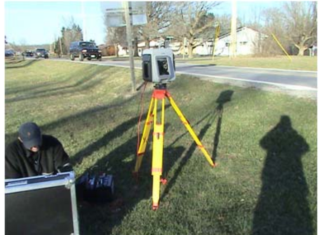
Static LiDAR Unit
