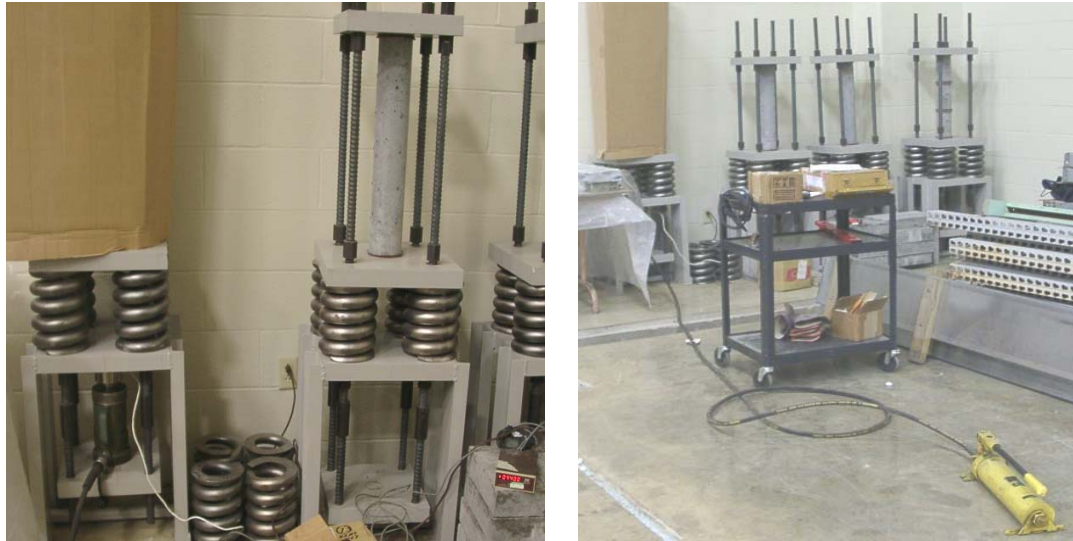
Figure 3.3 Creep Loading Frame and Specimens
