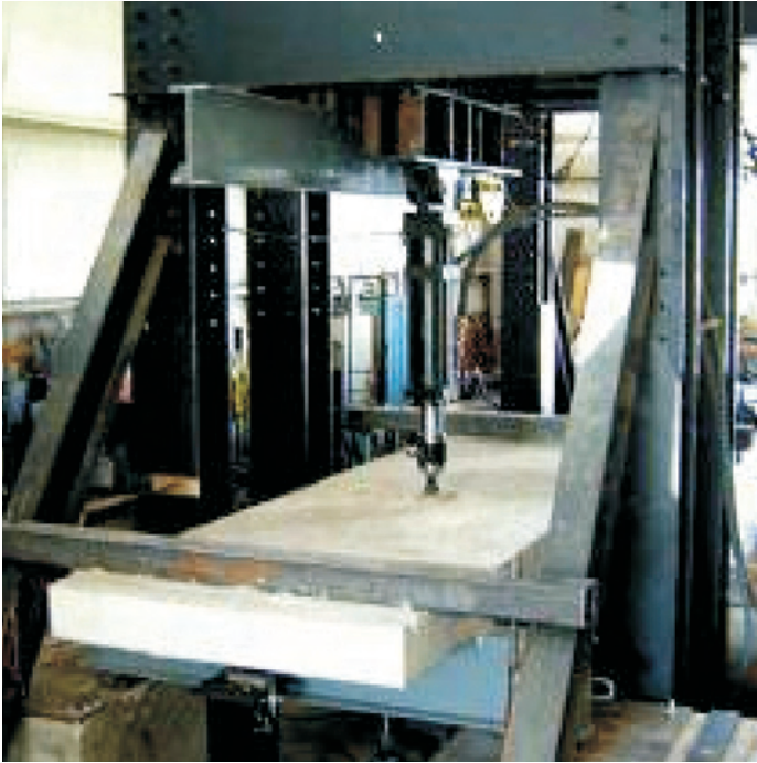
Fig. 2-Full-scale slab being subjected to static and fatigue loads
