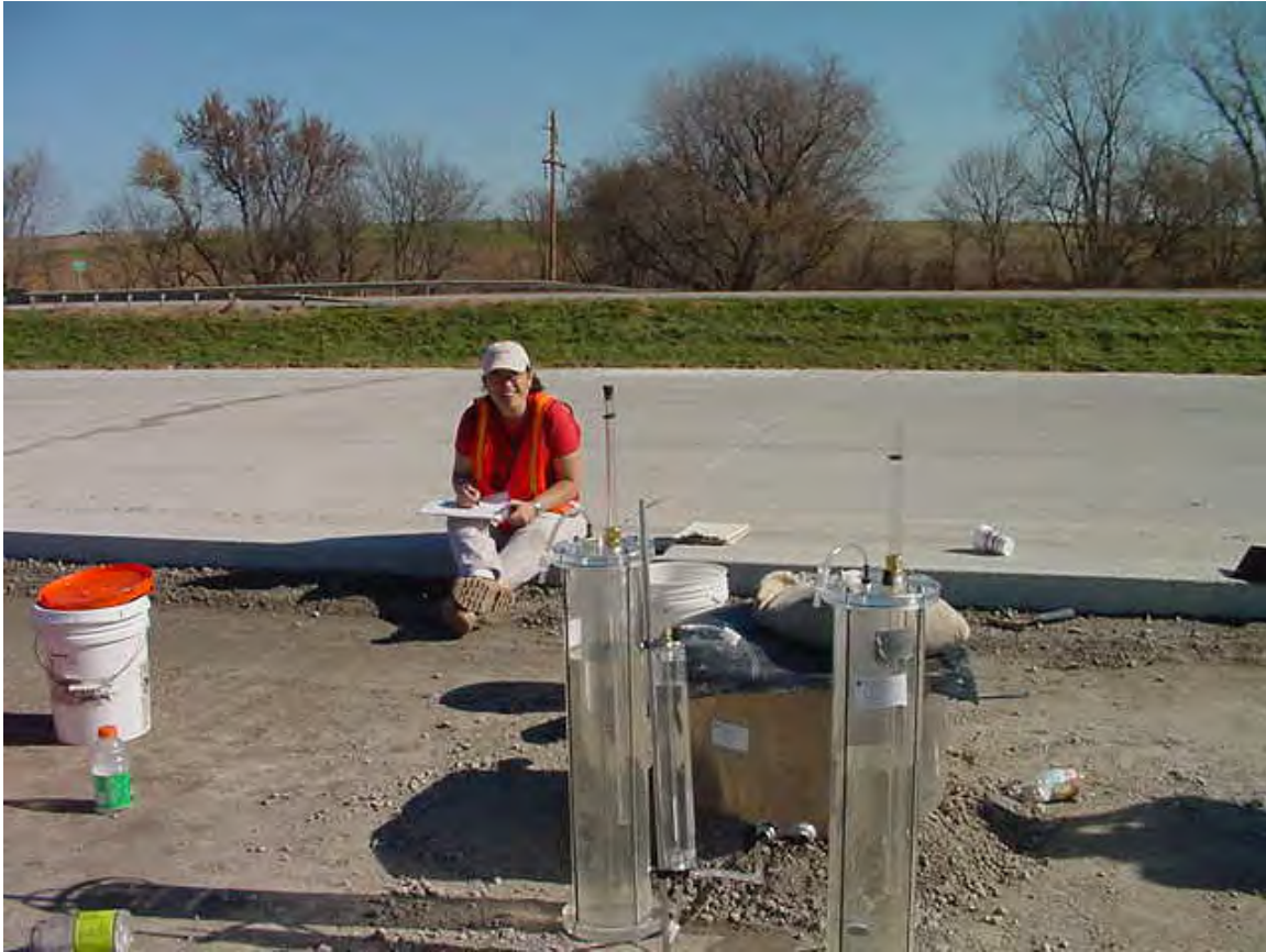
Figure 3 – Double ring infiltrometer
