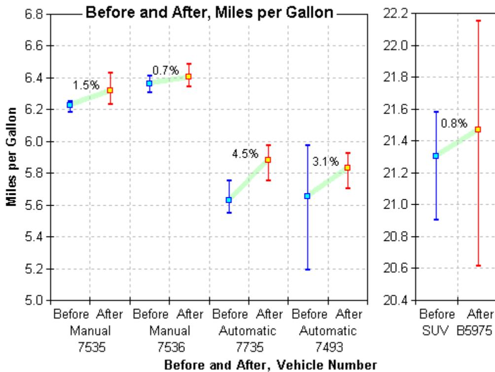
Figure 3, Graph of Minimum, Maximum, and Average Miles per Gallon Changes.
