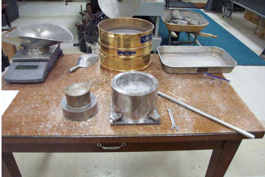
Figure 10: Missouri S&T ACV Mold, Rod, and Plunger
