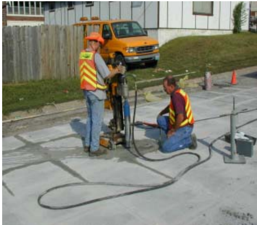
MoDOT Research personnel drilling cores for Iowa shears, SEM analysis, and pull off tests.
