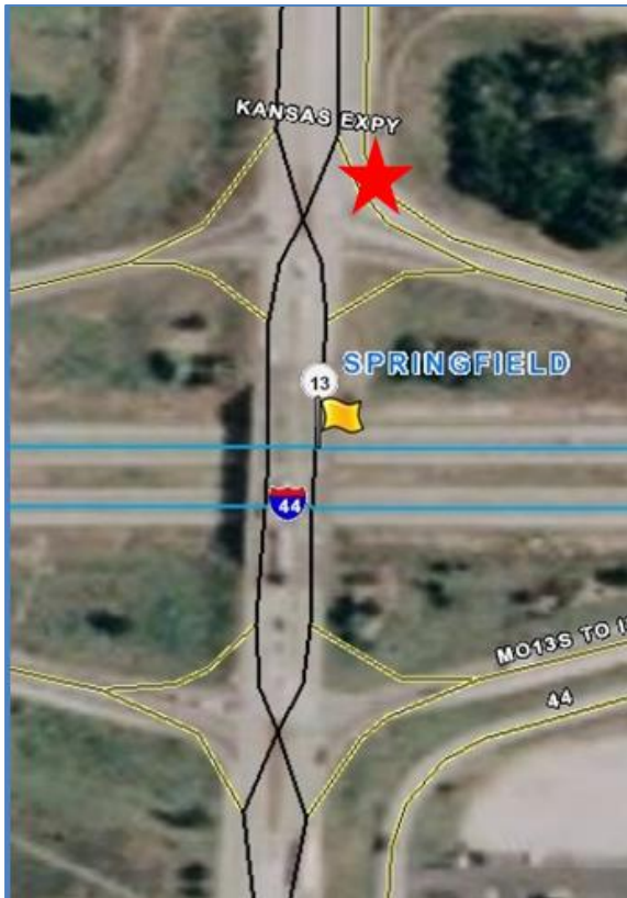
Example of Incorrect Crash Landing on Crossroad (Yellow Flag) and Correct Location on North Ramp (Red Star)
