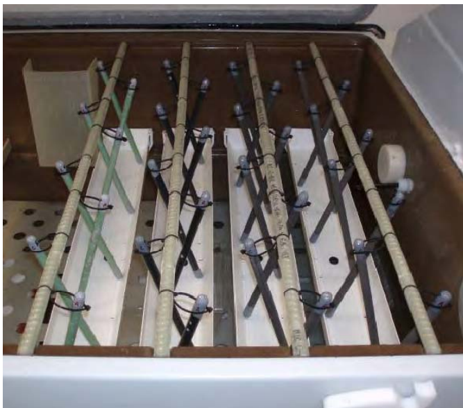
Wet phase testing of rebar coatings
