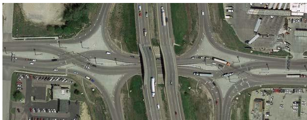
Aerial view of DDI at I-435 and Front Street, Kansas City, MO
