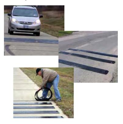
The safety industry already has taken notice. In February 2009, RoadQuake Temporary Portable Rumble Strips received a second place "Innovation Award" from the American Traffic Safety Services Association. Undoubtedly, further field testing is necessary to verify the positive results of the South Central districts field test. However, the value of RoadQuake temporary, portable rumble strips is clear.
