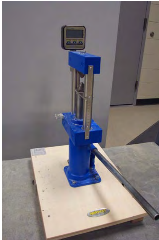
Figure 4: Point Load Device
