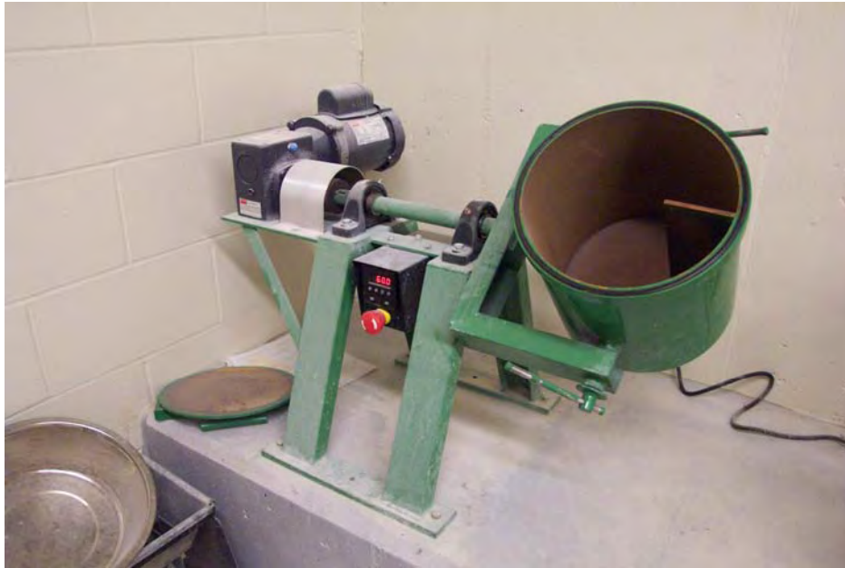
Figure 5: Wet Ball Mill Device
