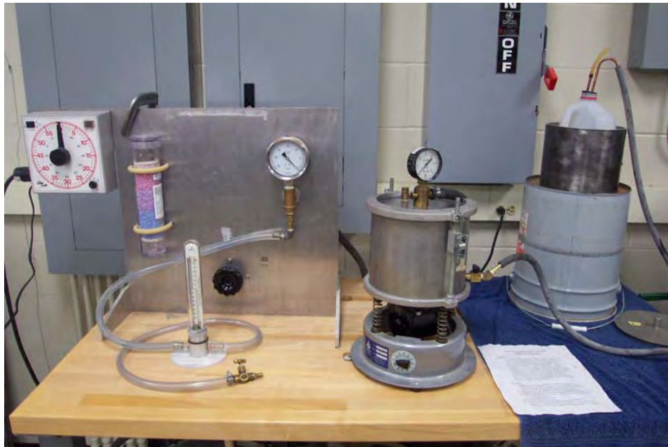
Figure 1: Vacuum Saturation Workstation
