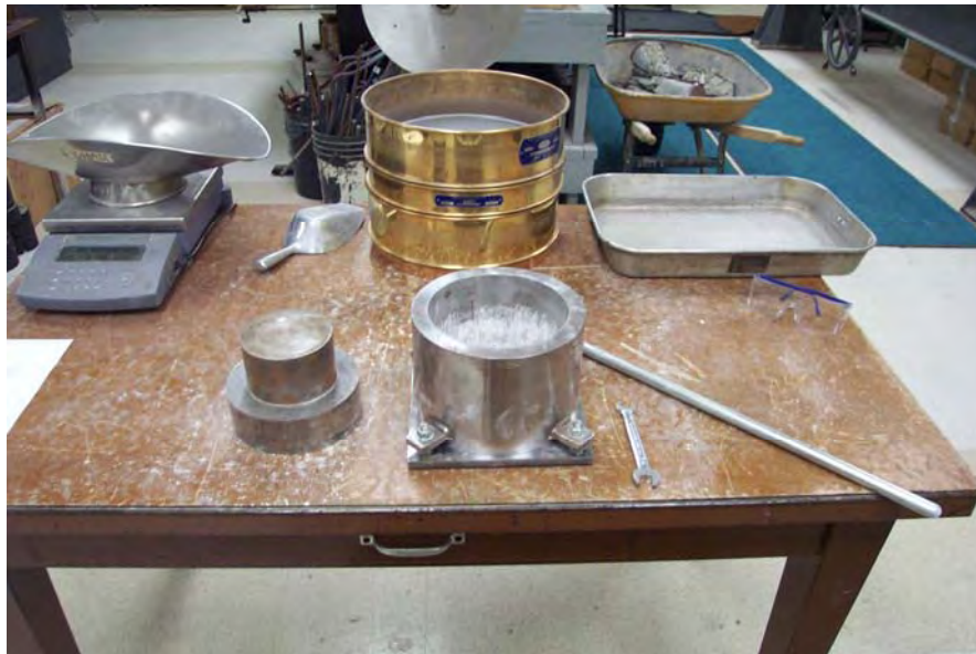
Figure 3: Missouri S&T ACV mold, rod, and plunger
